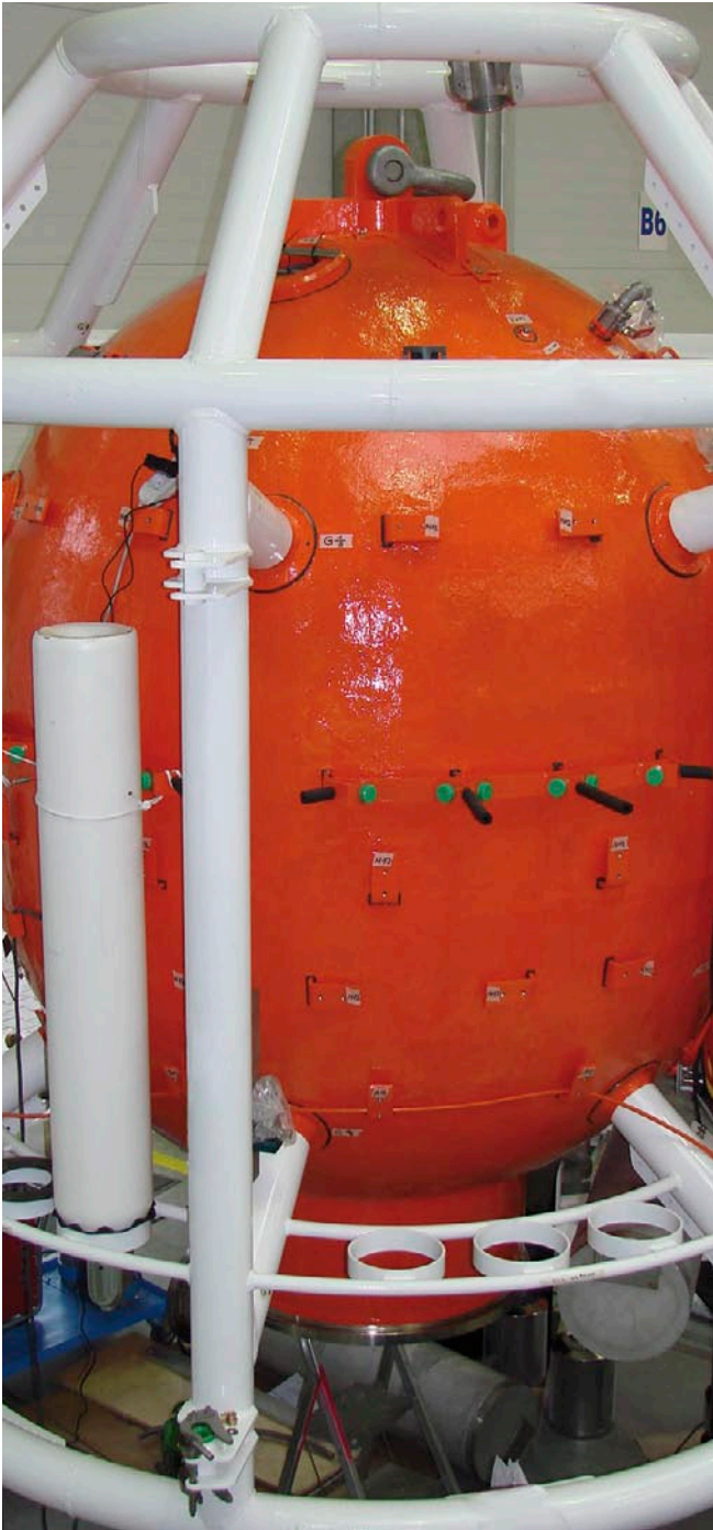
GL approved diving bell fitted for rough diving conditions
