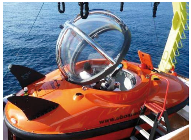
U-Boat Worx CQ3.1 Submersible, max. diving depth up to 100 msw
