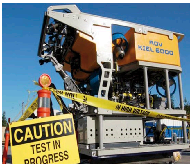
Heavy duty work class ROV, certified for 6000m diving depth
