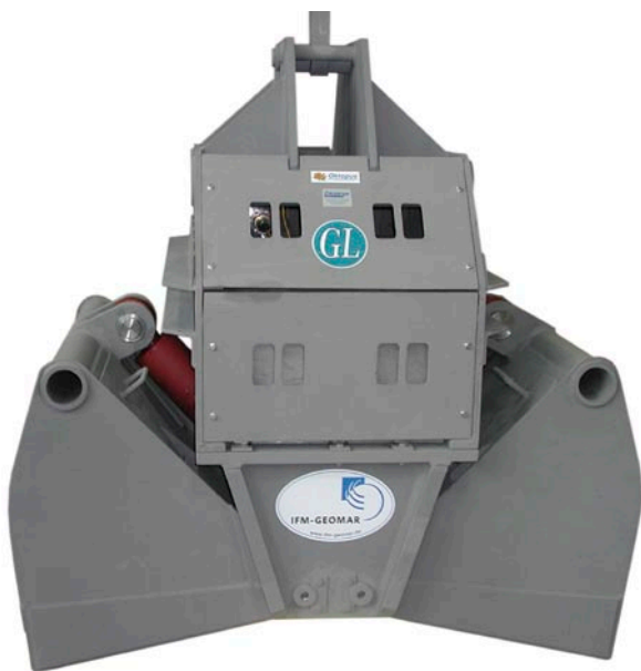
TV grab, underwater working device certified for 6000m diving depth
