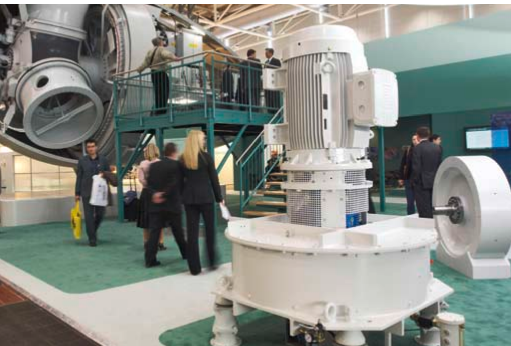
Flywheel energy storage system from Enercon.
