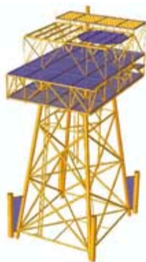
400 MW transformer offshore platform.
